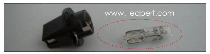
Then you just have to put the T5 Efficacity led in the original holder instead of the bulb and put the holder back on the meter. Do this for all the bulbs of your choice.
