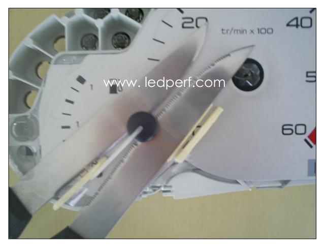
Once all the needles have been removed, remove the bottom of the meter to see which bulbs need to be changed.
