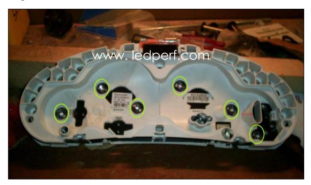
Step 7: Look at the back of the meter bottom in the light, to check if the meter bottom has a light layer of color or not. If the graduations are perfectly transparent, go directly to step 8. Otherwise, follow the instructions below.
